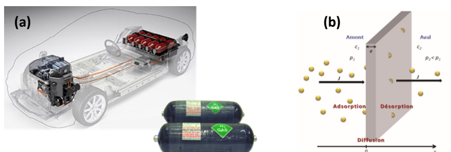
FIG1: (a) Hydrogen tank for automotiv sector. (b) The polymeric material using for the tank must have barrier properties to the H 2 gaz.
