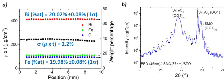
**Figure 2.** (a) Evolutions of density  $\times$  thickness product ( $\rho\cdot t$ ) and weight percentages of Bi, Fe and O as a function of the position and (b) X-Ray diffraction pattern of BFO/LSMO/STO heterostructure
