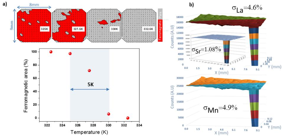
**Figure 6.** (a) Magnetic state maps of LSMO 20 uc film at various temperature (top) and  $T_c$  distribution at the sample surface (bottom). (b) WDS signal for La, Sr and Mn over  $9 \times 9 \text{ mm}^2$  of the same sample.
