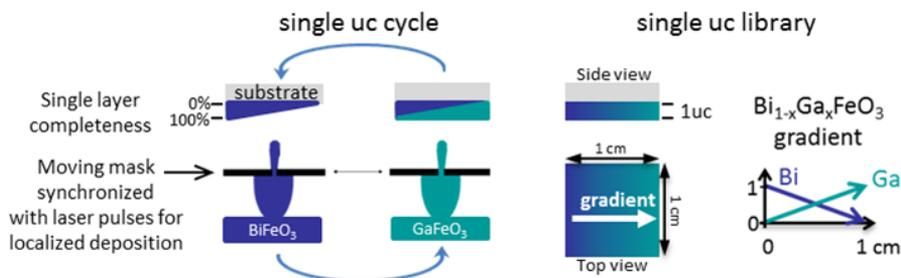
**Figure 1.** Schematic of the combinatorial single layer synthesis and of the resulting composition spread library (e.g.  $\text{Bi}_{1-x}\text{Ga}_x\text{FeO}_3$  composition library)
