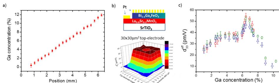
**Figure 3.** (a) Ga concentration measured by WDS along the composition gradient. (b) Heterostructure schematic (top) and  $d_{33}^{eff}$  mapping of a top electrode measured by laser vibrometry (bottom). (c) BGFO  $d_{33}^{eff}$  as a function of Ga content. From [18] with permission
