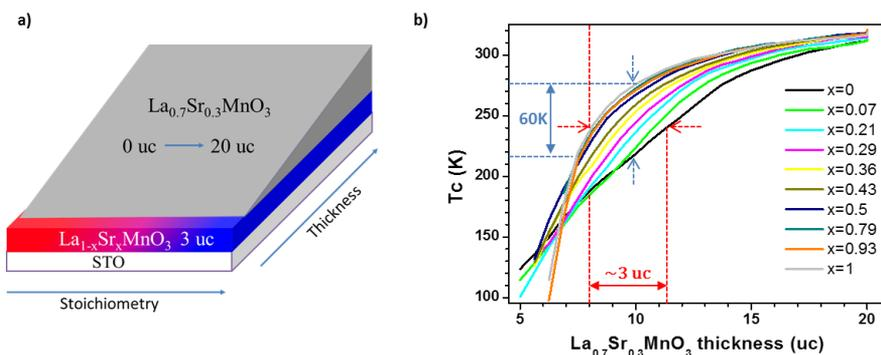
**Figure 8.** (a) Schematic representation of the ICPLD  $\text{LSMO}_x$  / wedge  $\text{LSMO}$  sample. (b) Curie temperature curves versus  $t_{\text{LSMO}}$  for various Sr content  $x$  in  $\text{LSMO}_x$  layer
