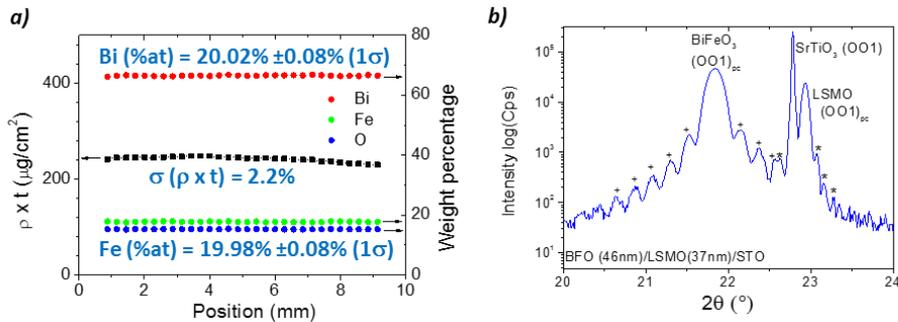
**Figure 2.** (a) Evolutions of density  $\times$  thickness product ( $\rho\cdot t$ ) and weight percentages of Bi, Fe and O as a function of the position and (b) X-Ray diffraction pattern of BFO/LSMO/STO heterostructure
